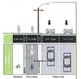
Figure 5: Design Concept for interim Cycle Track on Shelbourne Street
