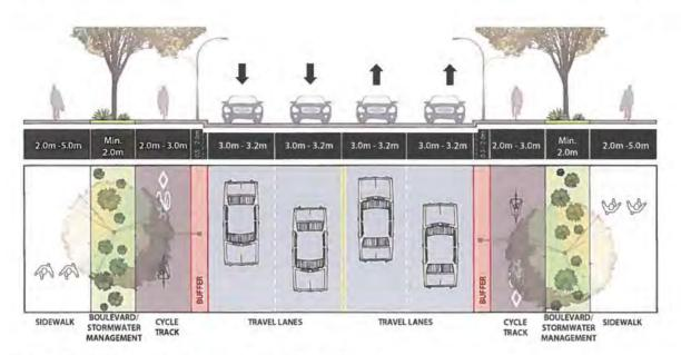
Figure 2: Mid-Term Shelbourne Street Right of Way
